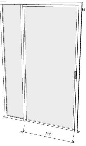
DOOR IS DELIVERED FULLY ASSEMBLED PLACE DOOR WITH INSIDE VERTICAL SUPPORTS AT 36" APART ALIGN DOOR TO BE SQUARE AND PLUMB EVEN IF RACKS ARE NOT
